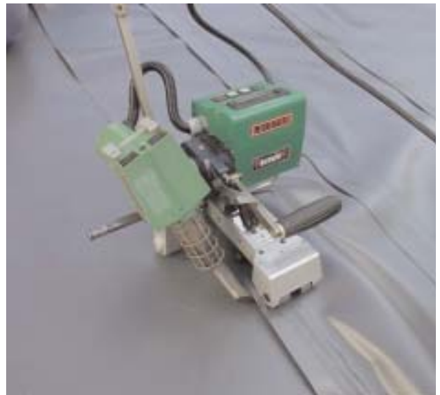
Photo 1a. Dual-track welding PVC geomembranes at TRI/Environmental in Austin, Texas.
