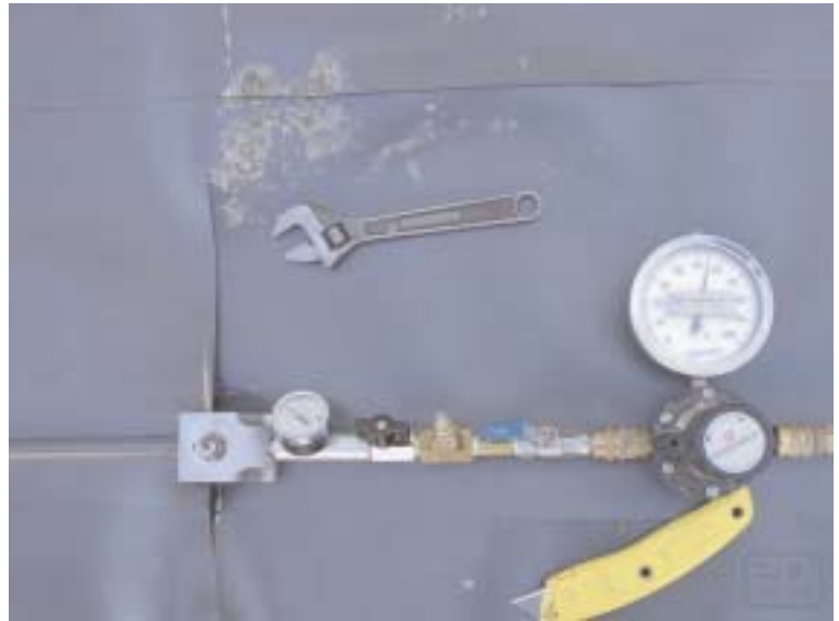
Photo 3. Seam burst test being performed.
