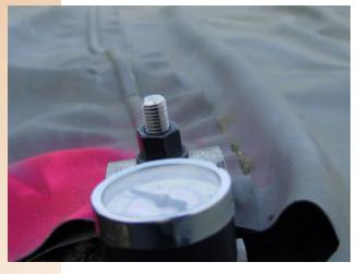
air channel testing. After completing two very large projects last fall using this technique to verify peel strength of field seams, EPI has a wealth of technical information on this process. If you are interested in learning more before the papers are published, just give us
