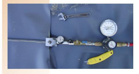
3 sections for peel testing and air channel testing at three different
