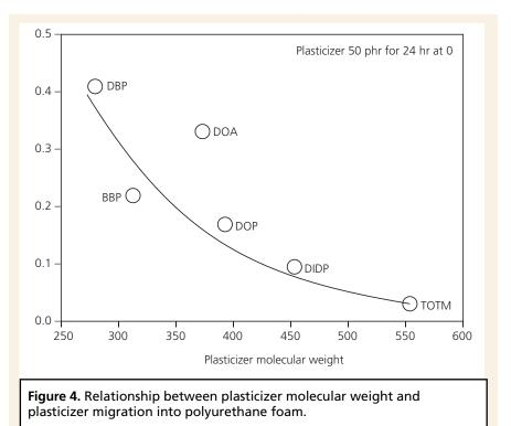
Figure 2 presents a relationship between molecular weight of common plasticizers and plasticizer loss by
