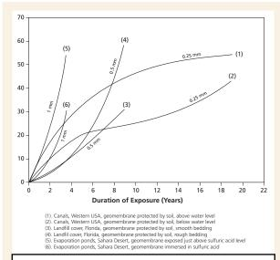
Figure 1. Plasticizer loss ratio versus duration of exposure (from Giroud and Tisinger 1993).
