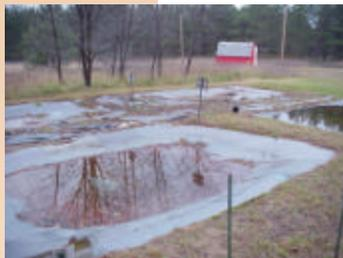
The material was installed on November 6, 1986, and left exposed to the weather since then. The samples of 20 mil were removed on November 2, 2001, almost 15 years to the day after installation. EPI will also be supplying Geoff with the test data and archived samples of the original material. These samples have been safely stored for 15 years at EPI waiting for just this opportunity. Geoff's testing of this material should yield valuable information on the durability of PVC geomembranes.
