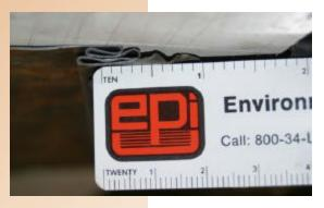
Folds in this liner material have been buried under 12" of sand cover and 10' of water since 1970 (more than 30 years). One sample of material
