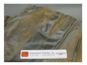
removal, samples exhibited the same flexibility as "NEW" PVC geomembrane. The flat areas of samples tended to be slightly less flexible after desiccation, but when folds in that material were unfolded, the material protected within the fold still exhibits the same flexibility as PVC liner material produced today! 30 years of solid performance shows that folds in PVC liner do not experience the
